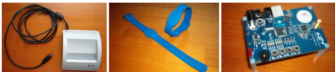
Fig. 3 A RFID reader (left), RFID wrist tags (center) and ZigBee development board (right) used in ALZ-MAS
