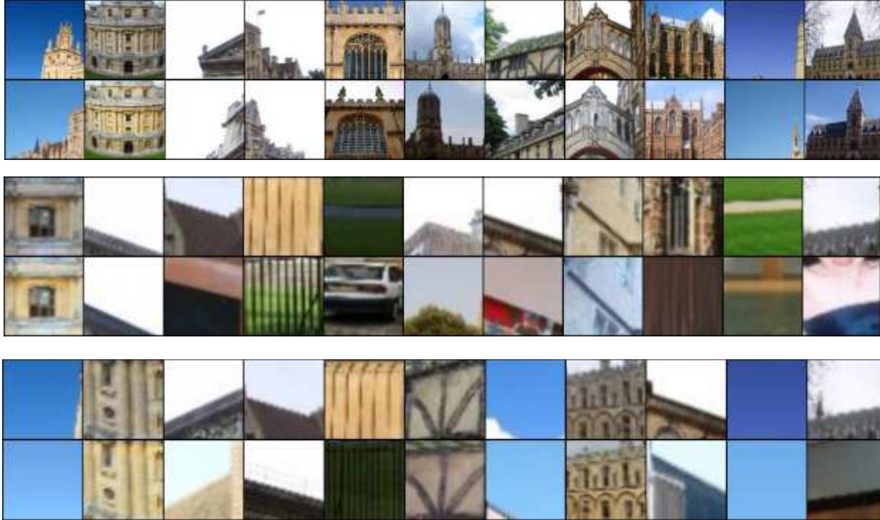
Figure 1. Randomly selected examples of image patches that are matched by individual deep features (top row), by original SIFT features (middle row) or by Fisher Vector-embedded SIFT features (bottom row). For deep features only the centers of corresponding receptive fields are shown. Overall, the matches produced by deep features has much lower false positive rate.
