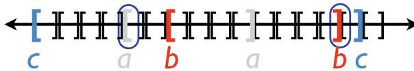
Fig. 7 An illustration of a partitioning query algorithm in action. The partition into alternative ranges is shown, along with three agents’ current bounding ranges, and the current median bounding range ( circled )
