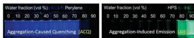
Fig. 1 Photographs of perylene (left) and hexaphenylsilole (HPS) solutions (right) with different poor solvent fractions taken under ultraviolet (UV) light irradiation.
