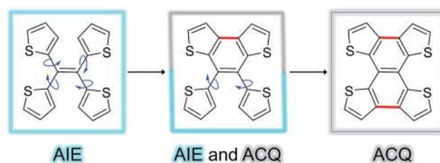
Fig. 5 Trend of the AIE phenomenon as a function of molecular structure. The blue arrows indicate the possible rotation of the thiophene rings around the single bond.
