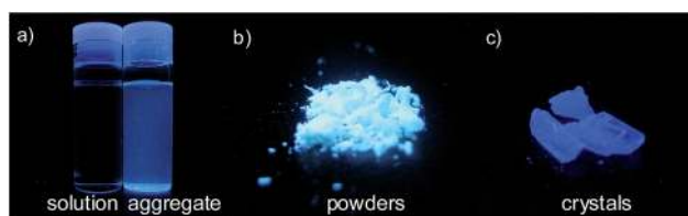
Fig. 3 Fluorescence photographs of (a) THF and aqueous solutions, (b) powders and (c) crystals of BS4, taken under the illumination of a UV lamp (365 nm). Reproduced with permission from ref. 25. Copyright (2013) Elsevier.
