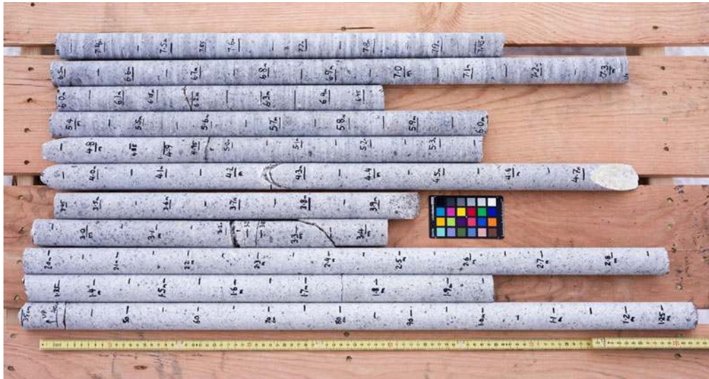
Fig. 17. Granite bedrock core recovered from Site 2 during the 2016–17 Pirrit Hills, Antarctica field project. Both the PDC and diamond-impregnated bits produced similar quality core.
