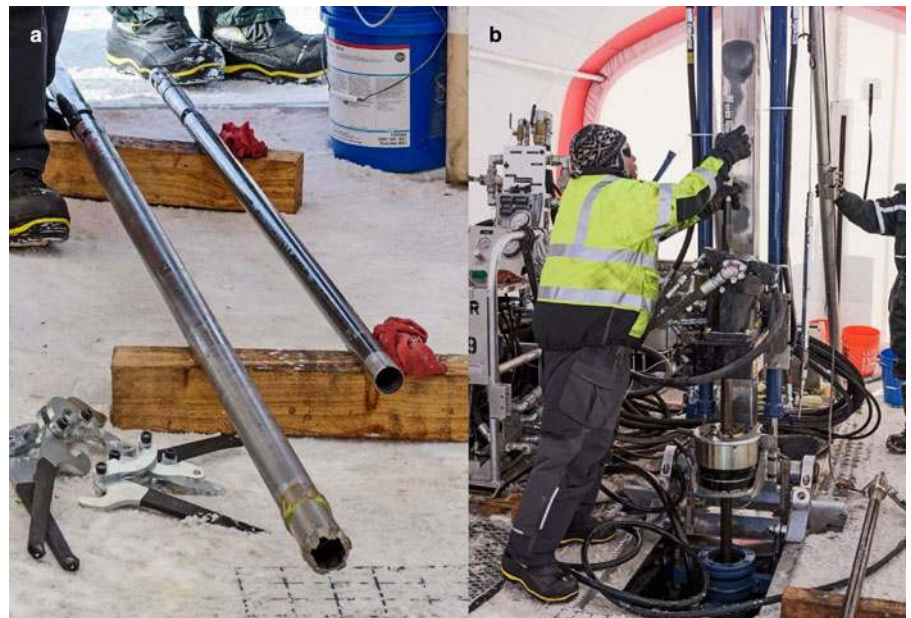
Fig. 7. (a) BHA with coring bit and rock reaming shell (left) and inner core barrel assembly (right). (b) Deploying the inner core barrel assembly into the drill pipe string.
