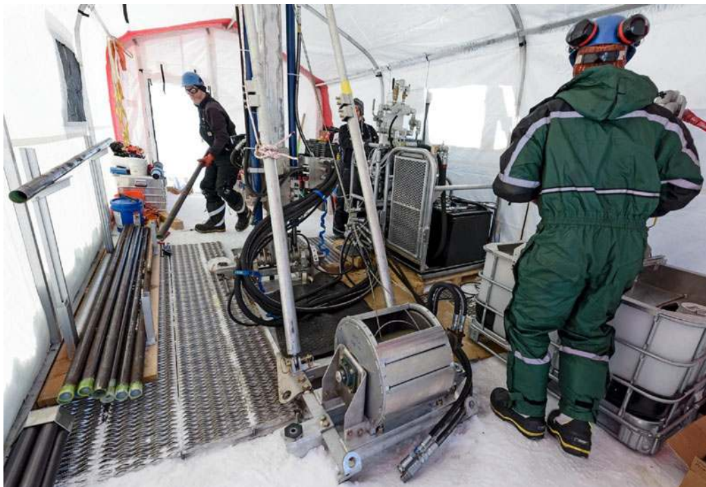
Fig. 16. Access hole drilling operations with the ASIG Drill system at Site 1 during the Pirrit Hills, Antarctica field project in 2016.
