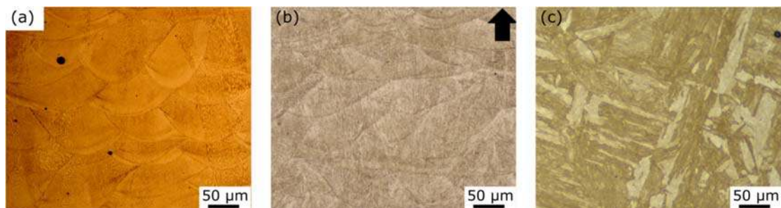
Figure 2. Optical micrographs of the printed and heat treated samples. a) in the as printed condition, b) aged at 480 \text{ }^\circ\text{C} for 1 h and c) solution treated at 850\text{ }^\circ\text{C} and aged at 480 \text{ }^\circ\text{C} for 6 h. The arrow indicates the common building direction.
