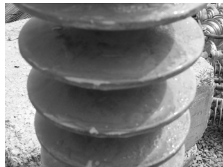
Figure 5. Dirty sheds. Nearest the camera are regions of crazed surface. The light areas at the very front were probably cleaned off during removal of the insulator from the tower.
