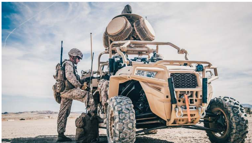
Figure 3.1. Light Marine Air Defense Integrated System Jammer Mounted on Polaris MRZR Vehicle
