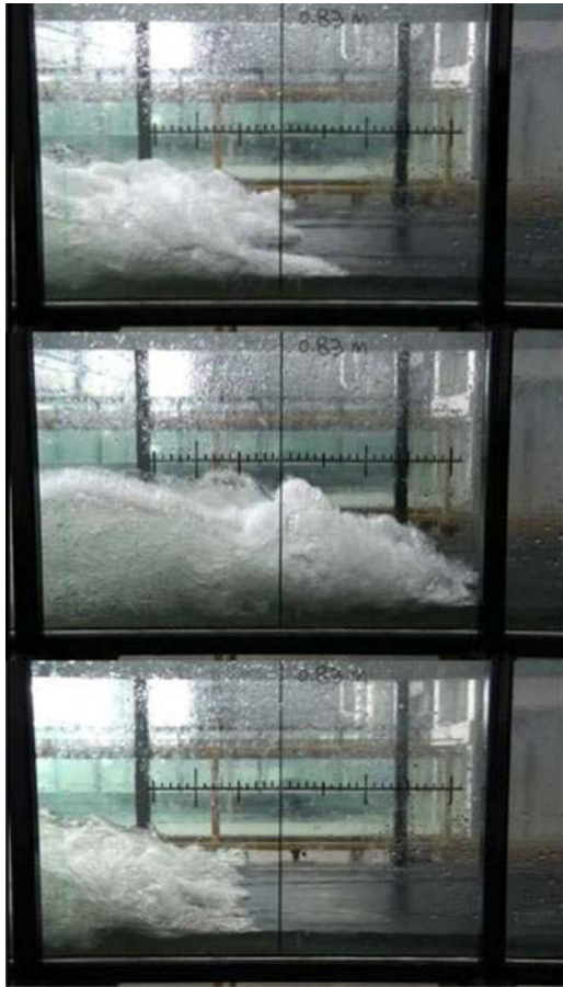
Figure 11. Video frames of hydraulic jump toe position in side view.
