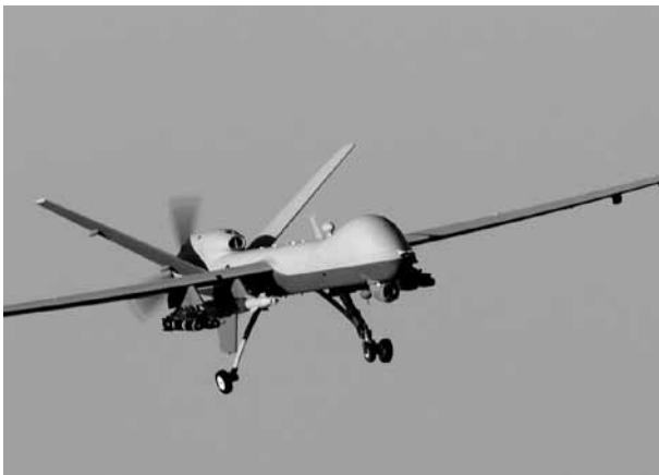
A General Atomics Aeronautical Systems MQ-9 Reaper with its armament intact after a combat sortie in Afghanistan. (USAF photo/SSgt. Brian Ferguson)
