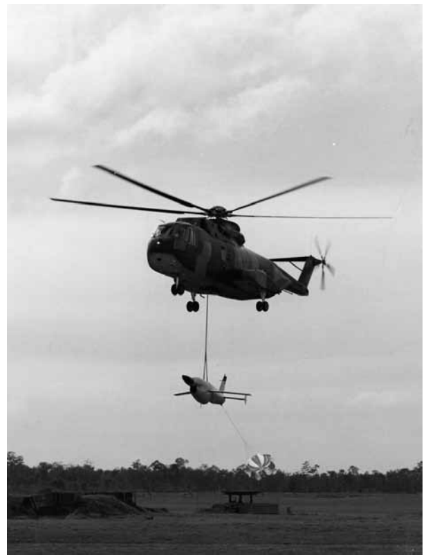
A CH-3 helicopter returns to home base after recovering an AGM-34 RPV.
