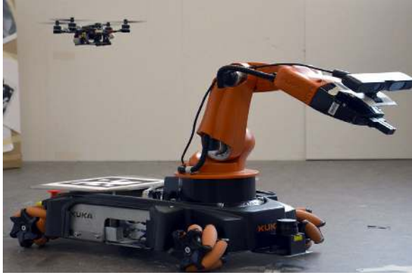
Fig. 16: The NanoQuad MAV, equipped with a down-looking camera and an onboard computer, is hovering above the Kuka YouBot ground robot, equipped with an RGBD camera.
