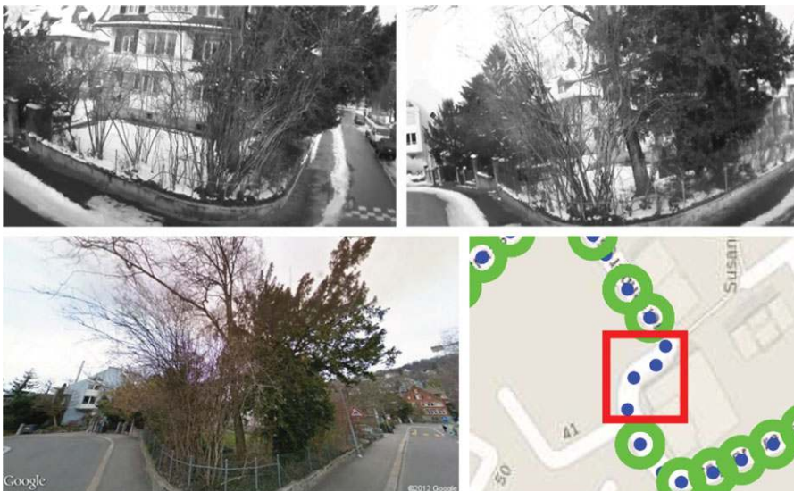
Figure 19. Analysis in case of no detections. Top-left: urban MAV image; top-right: next view of the urban MAV; bottom-left: true positive pairing according to manual labeling; bottom-right: zoom on the global map, where the image was taken. Please note that these robot positions (top row) are difficult to recognize even for humans. Moreover, the over-season change of the vegetation makes it extremely difficult to cope with their pairing for image feature-based techniques.
