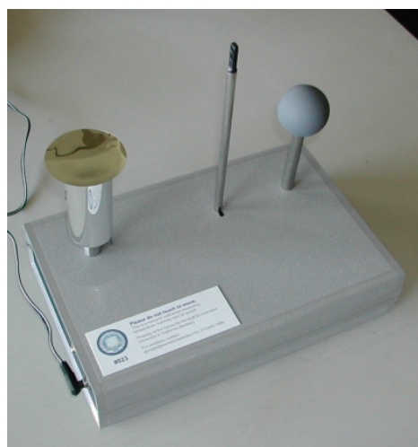
Figure 2b. Desktop weather station with (from left to right) shielded dry bulb sensor, anemometer, and globe temperature sensor
