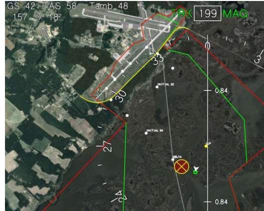
Figure 11. Image of MOS Range Display, showing navigational information and predicted impact point information relative to operational and range boundaries.
