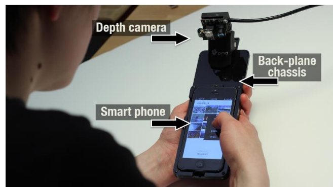
Figure 3. Our prototype smart phone uses a depth camera to simulate future, more advanced hover-capable devices. We used this setup as a vehicle for exploration and also as a platform to develop several Air+Touch augmented applications.
