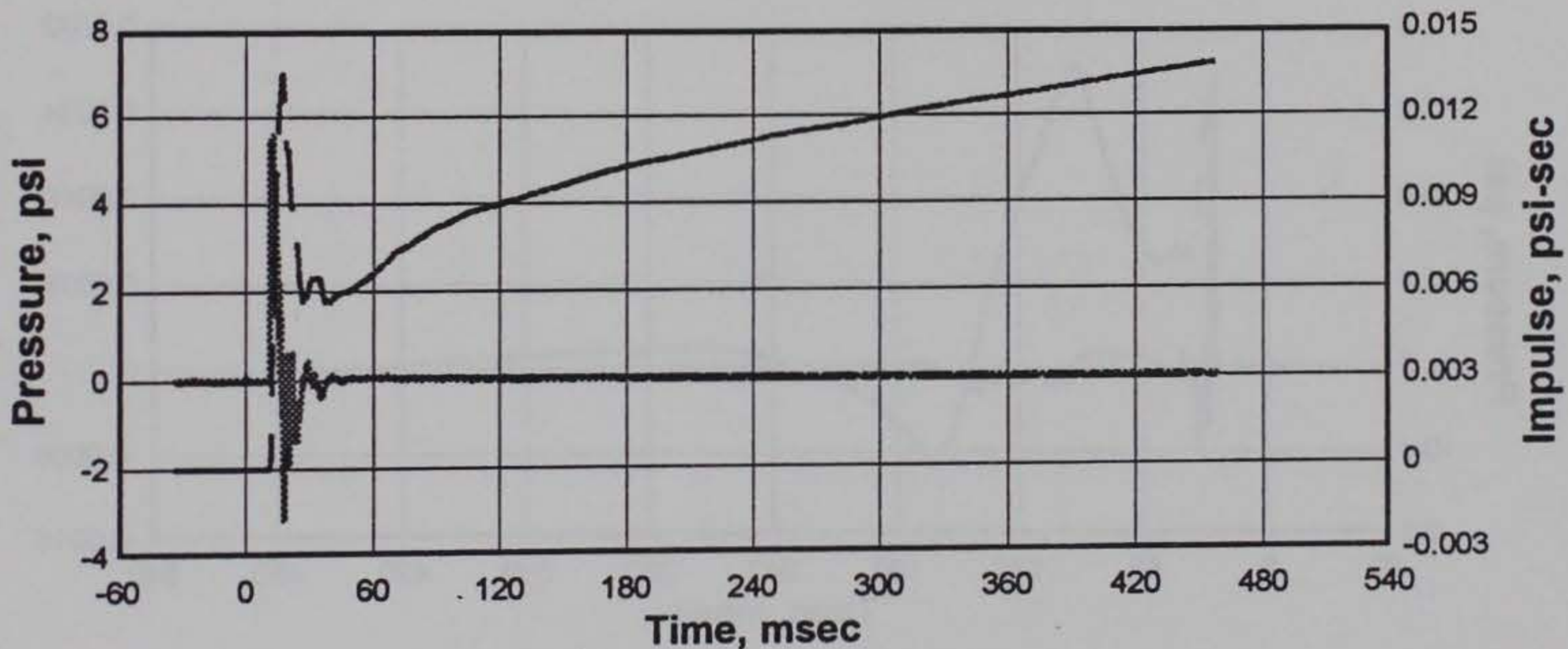
Figure C12. Pressure and impulse-time histories, free-field Gage AB-13 on surface of the ground at a horizontal distance of 3.00 m from the portal, Experiment 3.
