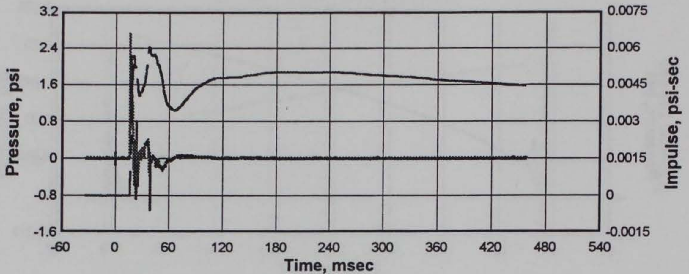
Figure B13. Pressure and impulse-time histories, free-field Gage AB-15 on the surface of the ground at a horizontal distance of 4.80 m from the portal, Experiment 2.
