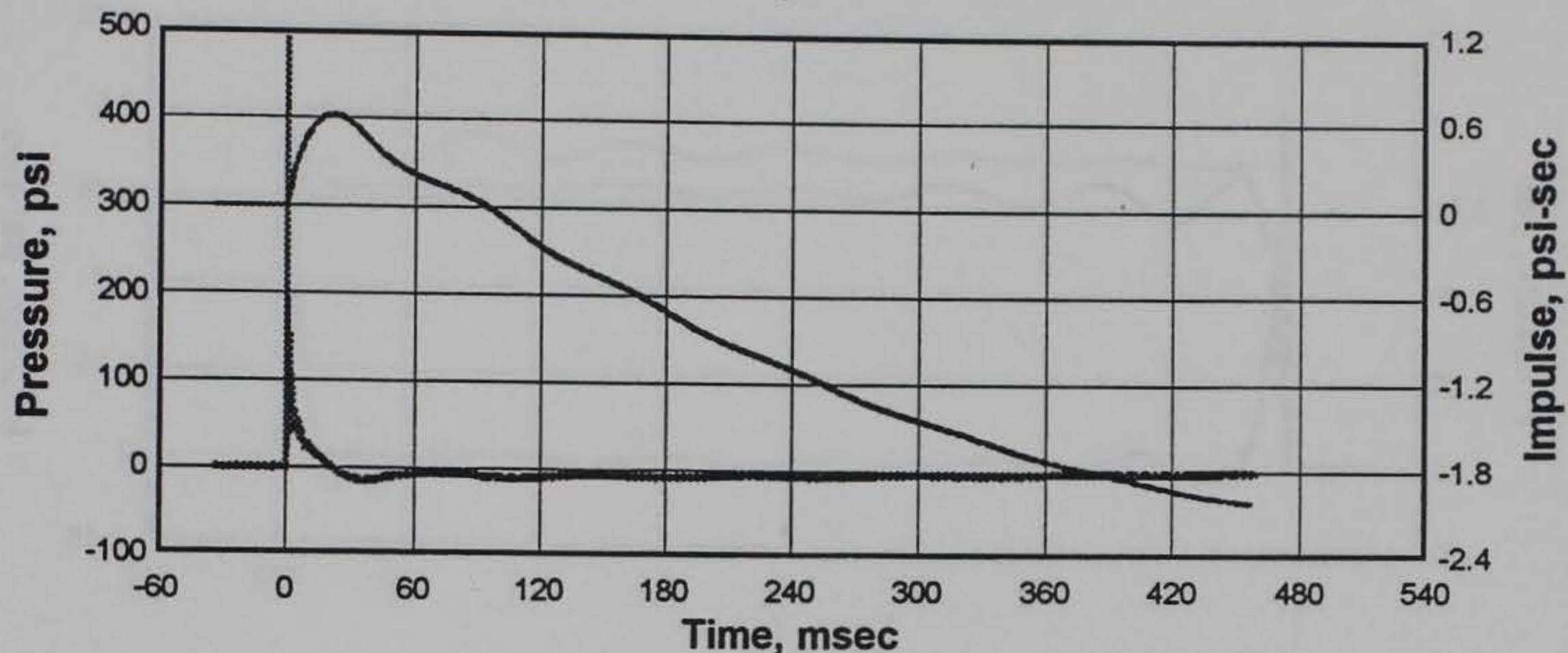
Figure B3. Pressure and impulse-time histories, Gage AB-3 on the side wall of the detonation chamber at a horizontal distance of 1.35 m from the rear wall of the detonation chamber, Experiment 2.
