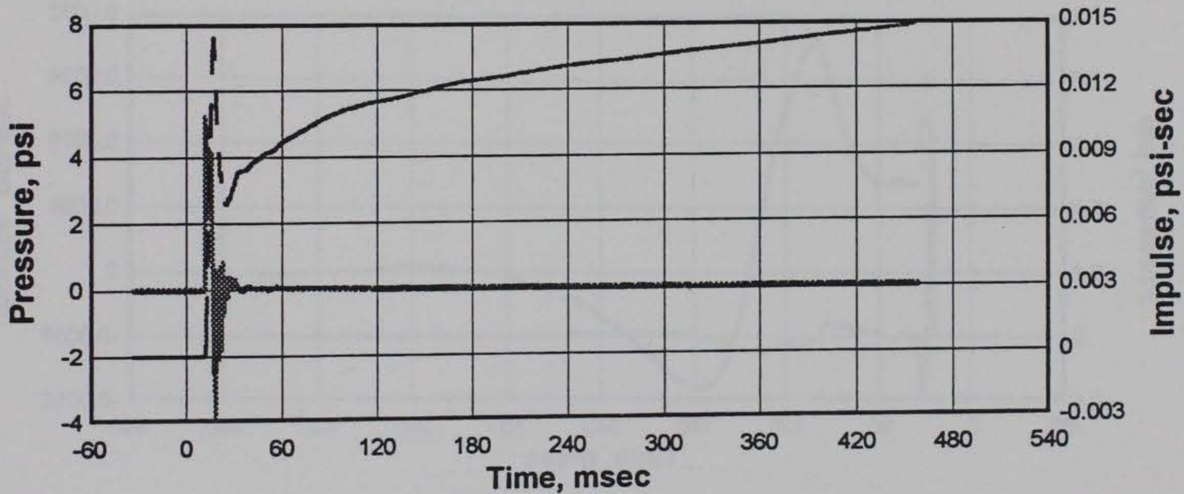
Figure A12. Pressure and impulse-time histories, free-field Gage AB-13 on the surface of the ground at a horizontal distance of 3.00 m from the portal, Experiment 1.
