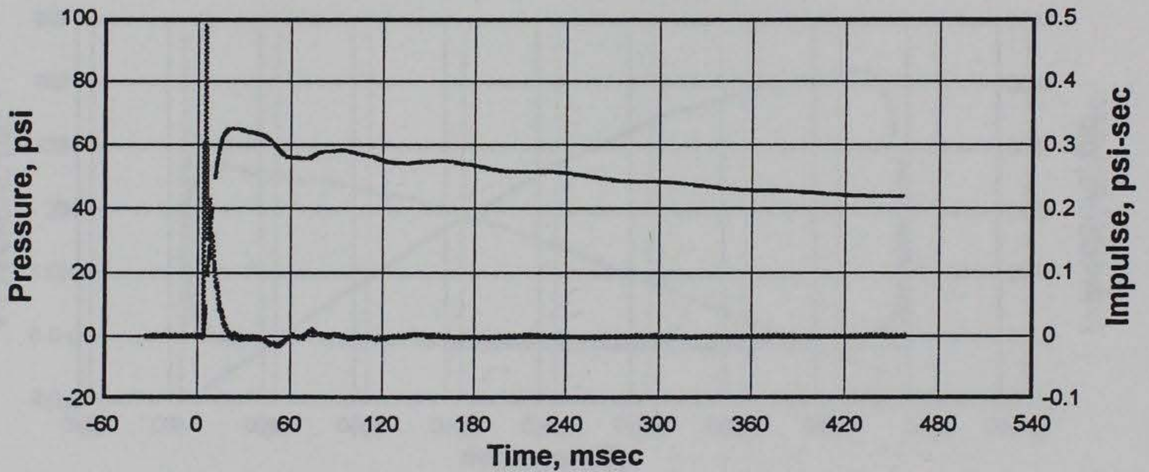
Figure A10. Pressure and impulse-time histories, Gage AB-11 on wall of the access tunnel at a horizontal distance of 5.61 m from the rear wall of the detonation chamber, Experiment 1.
