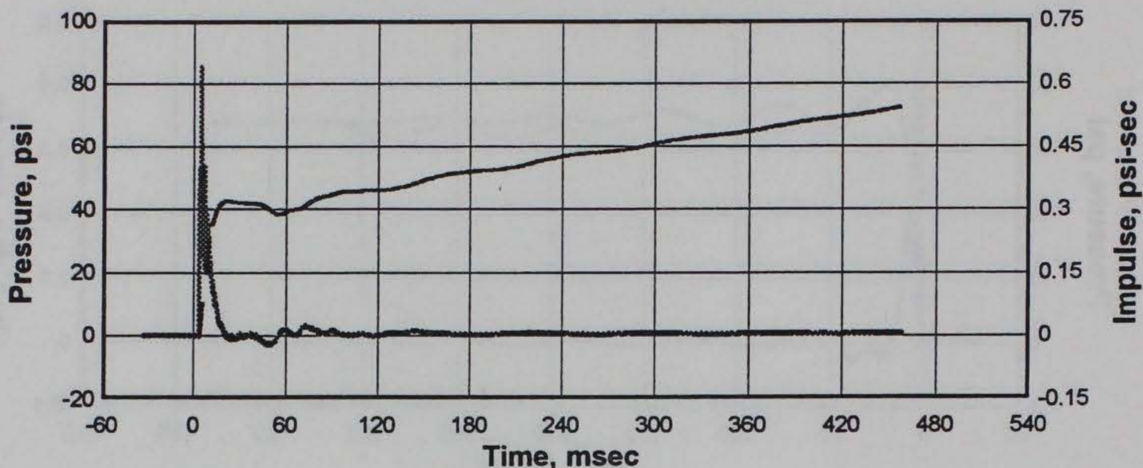
Figure C9. Pressure and impulse-time histories, Gage AB-10 on wall of access tunnel at a horizontal distance of 5.30 m from the ear wall of the detonation chamber, Experiment 3.
