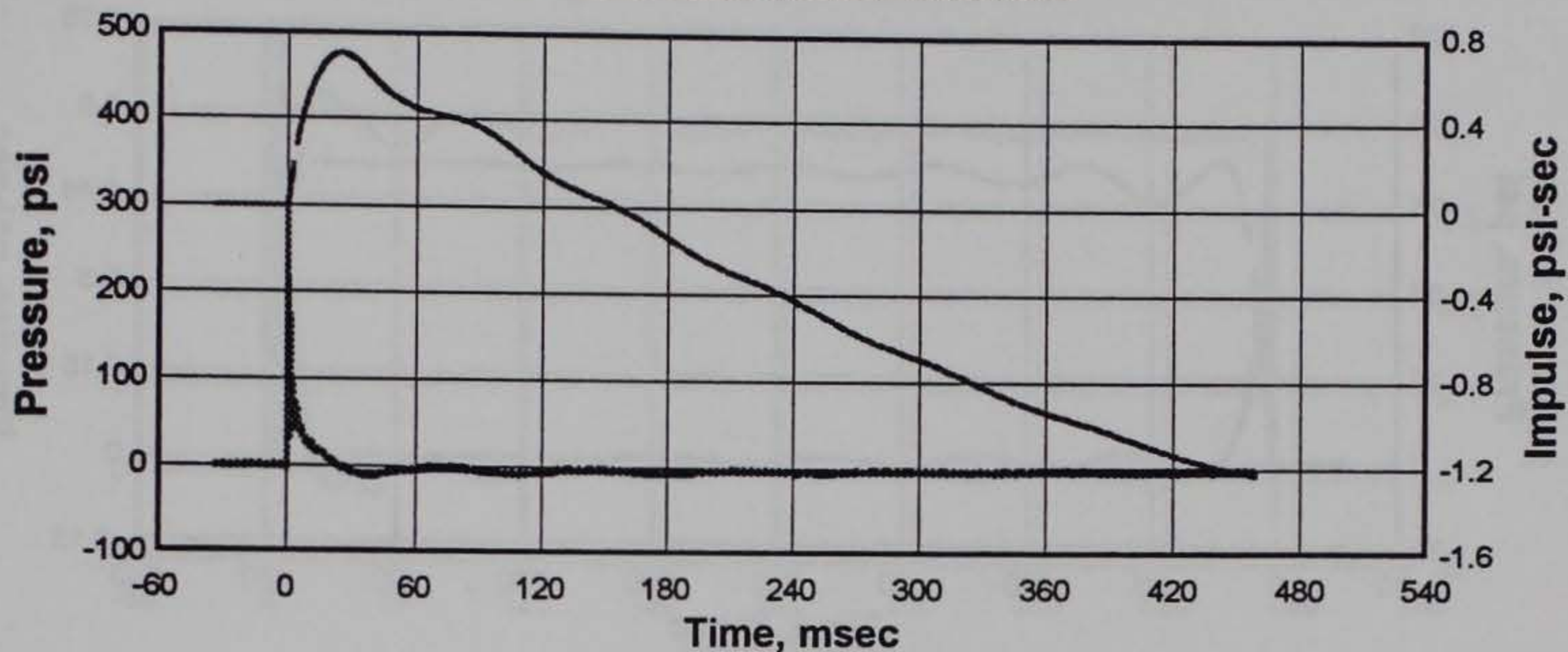
Figure A3. Pressure and impulse-time histories, Gage AB-3 on side wall of the detonation chamber at a horizontal distance of 1.35 m from the rear wall of the detonation chamber, Experiment 1.
