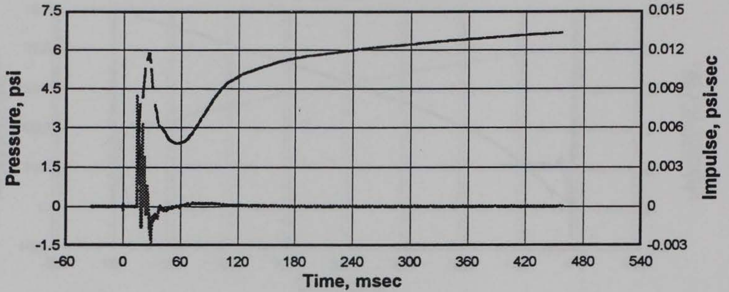
Figure D13. Pressure and impulse-time histories, free-field Gage AB-15 on surface of the ground at a horizontal distance of 4.80 m from the portal, Experiment 4
