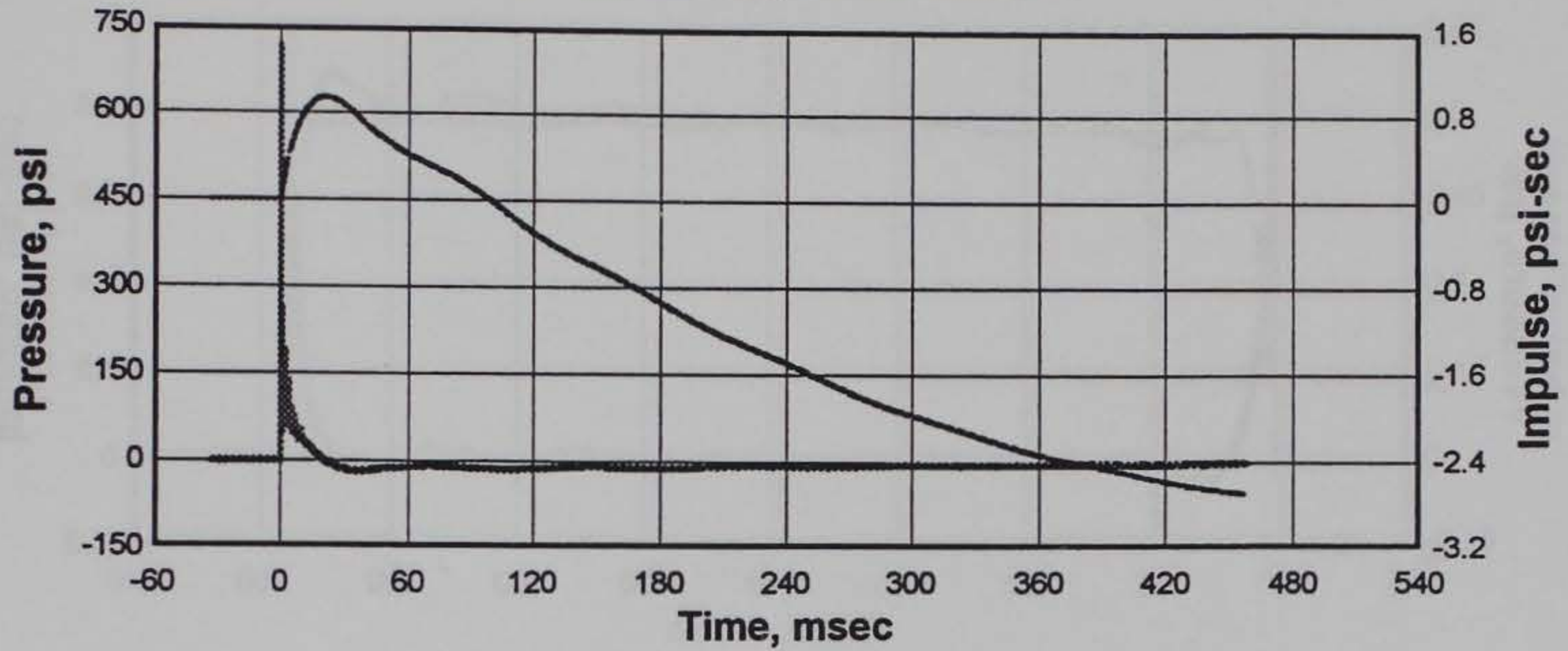
Figure D3. Pressure and impulse-time histories, Gage AB-3 on side wall of the detonation chamber at a horizontal distance of 1.35 m from the rear wall of the detonation chamber, Experiment 4.
