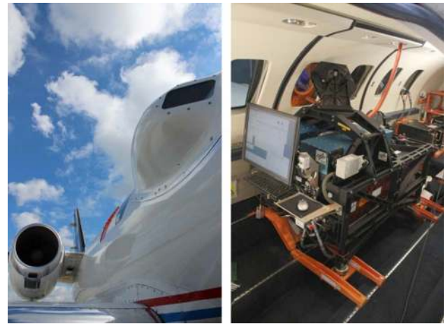
Fig. 2. Left: view on the outside starboard fuselage with the fairing for laser beam transmission and reception. Right: complete lidar and beam steering system with operator interface.
