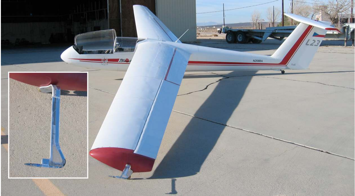
Figure 3. U.S. Air Force Test Pilot School Super Blanik L-23 sailplane with wingtip-mounted microphone; closeup of microphone shown in inset.
