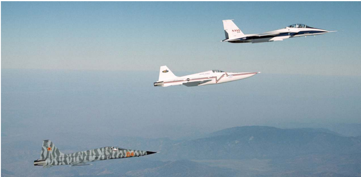
Figure 1. SSBD aircraft (Northrop Grumman), center, F-15B-836 aircraft (NASA Dryden), upper right, baseline F-5E (U.S. Navy Fallon NAS), lower left.
