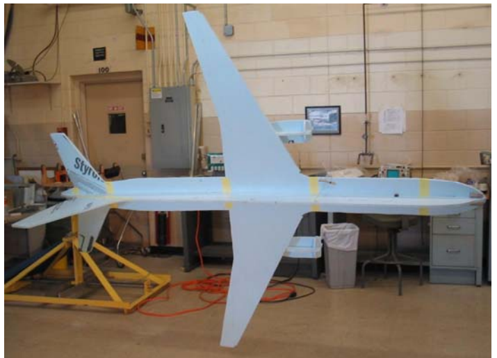
Figure 10. 5.5% GTM-ADM undergoing pitch testing
