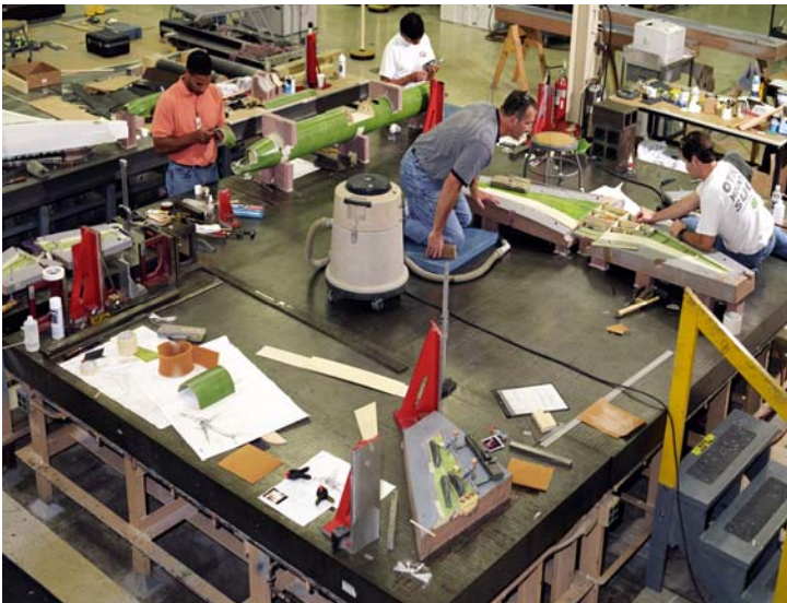
Figure 5. The 5.5% GTM-T1 under construction
