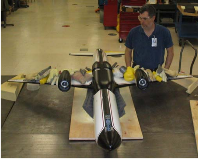
Figure 7. 5.5% GTM-T1, positive direction proof loading with a total of 195.21 lbs
