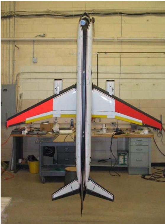
Figure 9. GTM-T1 undergoing roll inertial testing at full fuel.
