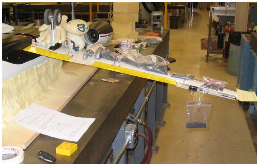
Figure 8. Left aileron load test with positive deflection.
