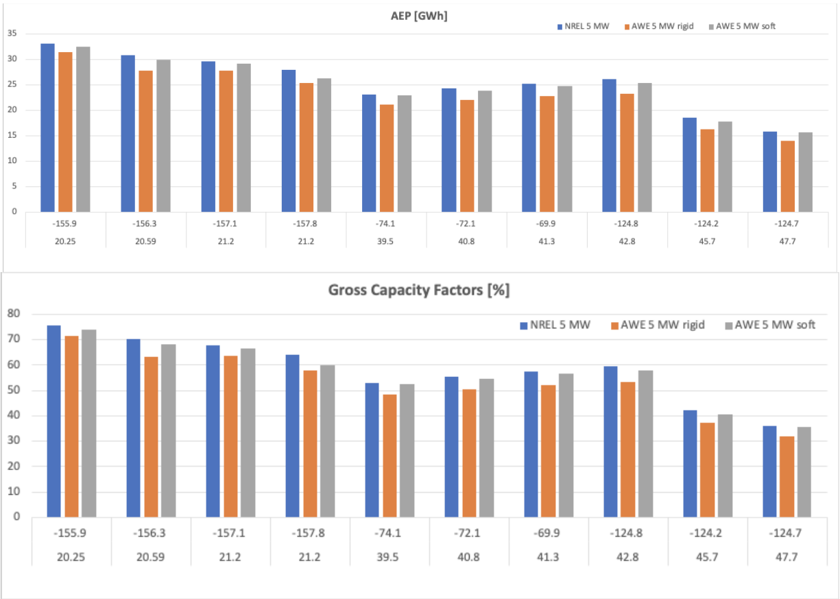
Figure 21. (top) AEP estimates and (bottom) gross capacity factor (averaged over 20 years) for selected locations offshore (indicated by longitude/latitude, see Figure 12). The calculations assume 100% availability.
