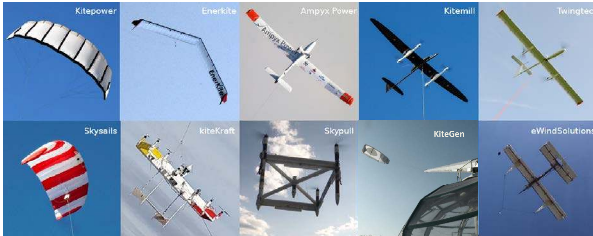
Figure 5. AWE system prototypes currently under development (in flight). Images based on Schmehl (2018)
