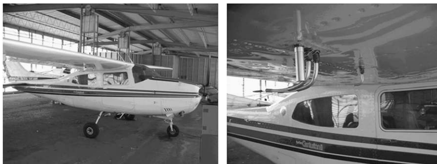
FIG. 3. The Cessna T210 used in light aircraft flights. Right photo shows inlet locations.
