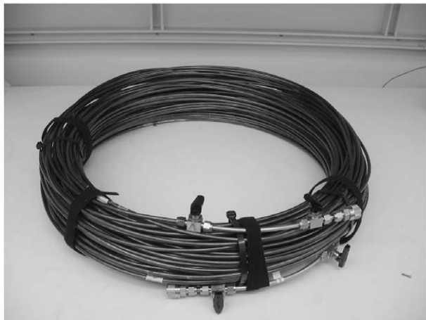
FIG. 1. The AirCore with magnesium perchlorate driers and shut-off valves attached on each end.
