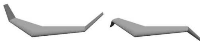
Fig. 12 Baseline, symmetric configurations for pitch control.
