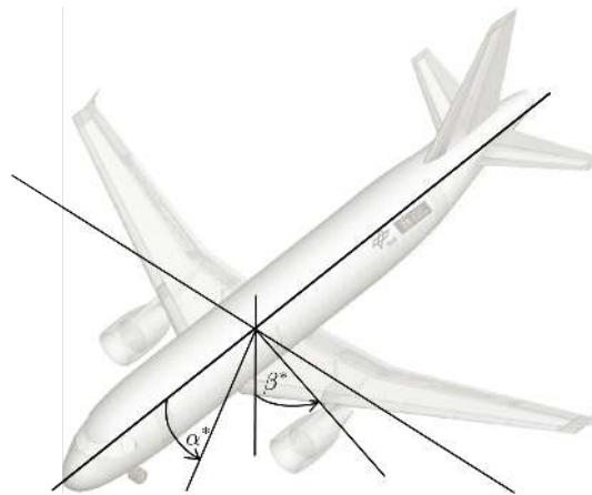
Figure 14. Definition of the emission angles \alpha^* and \beta^* .
