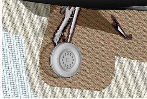
Figure 3 Volume mesh in the vicinity of main gear and flap showing different resolution levels.
