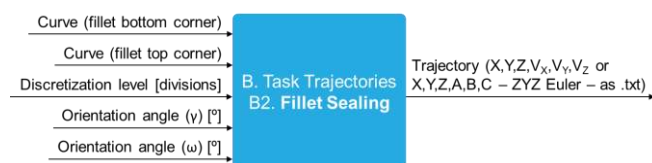
Fig. 13: Inputs and outputs of the algorithm for generation of fillet in sealing task trajectories.
