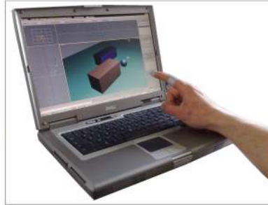
Fig. 6 Left: Use of the two hands for 3D rotation: metaphor of planting a pin inside the object to be rotated. Right: Mixed 2D and 3D Interaction with AirMouse in Autodesk 3D Studio Max. the 2D pointing technique has been plugged to the mouse cursor while 3D pointing becomes active when the user moves over the perspective 3D view.
