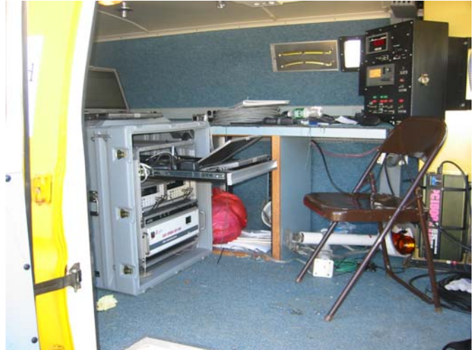
Figure 5 – The FAATC test van employed for ground data collection.
