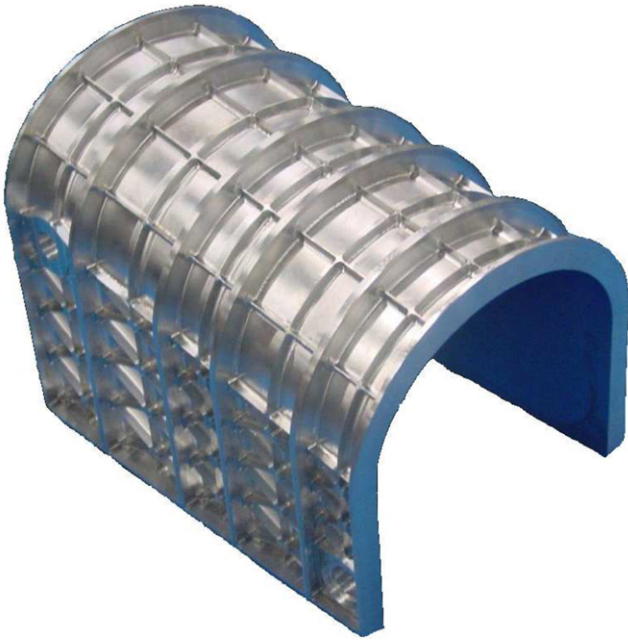
Fig. 10. Manufactured prototype of the landing gear compartment. The studied parts are the inner surfaces of the structure.
