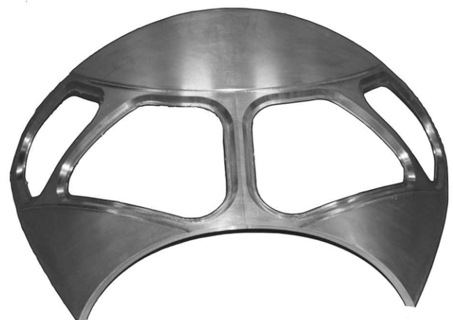
Fig. 9. Manufactured prototype of the cockpit.
