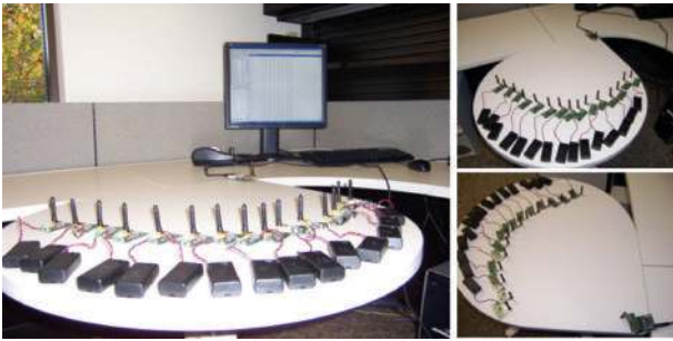
FIGURE 9: Experiment setup number 2: nodes on a table close to base station.
