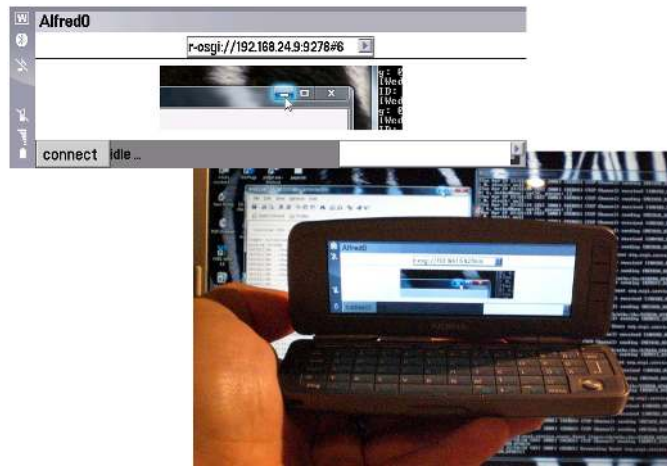
Fig. 7. MouseController running on a Nokia 9300i phone
