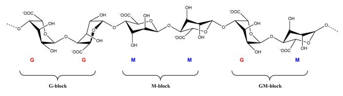
Figure 2. Chemical structure of alginate.
