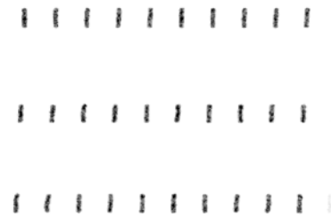
Figure 4: A portion of a slit image taken using the COS flight detector. The slits are 25 \times 500 \mu\text{m} on 200 \mu\text{m} centers. Each row is separated by 2.5 mm.
