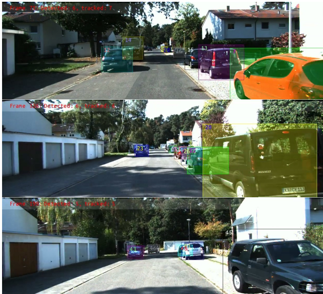
Figure 4.4: Sample tracking results on KITTI dataset sequence ‘0007’, targets are marked with colored rectangles and with numbered ID (better view in color).
