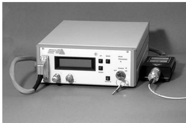
Figure 2.7: PIL040G 408 nm laser.
