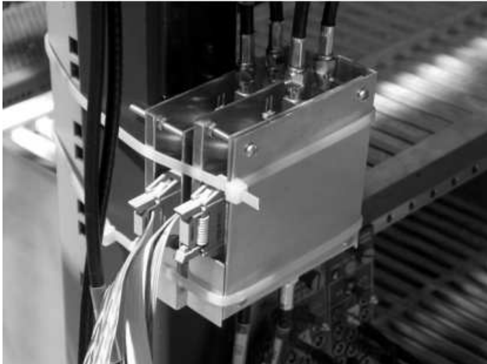
Figure 2.43: Photograph of the shoebox prototype (for two input channels) tested at CERN PS in June 2004. The input cables are seen entering from below and the output cables exit from the top. The ribbon cables deliver \pm 6\text{V} of power.
