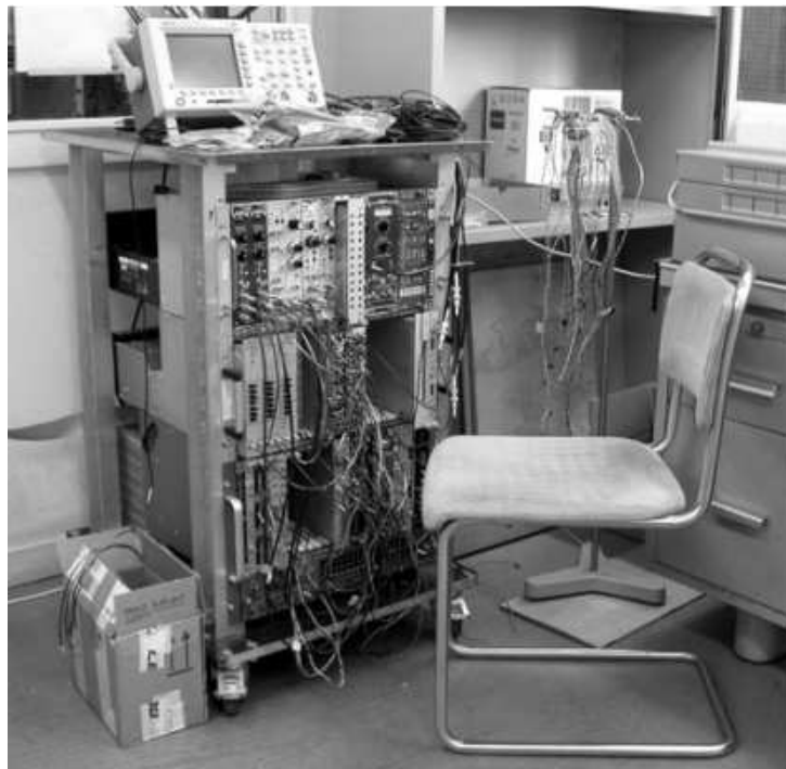
Figure 2.44: Test version of the main T0 electronics rack photographed during the 2004 run at CERN.
