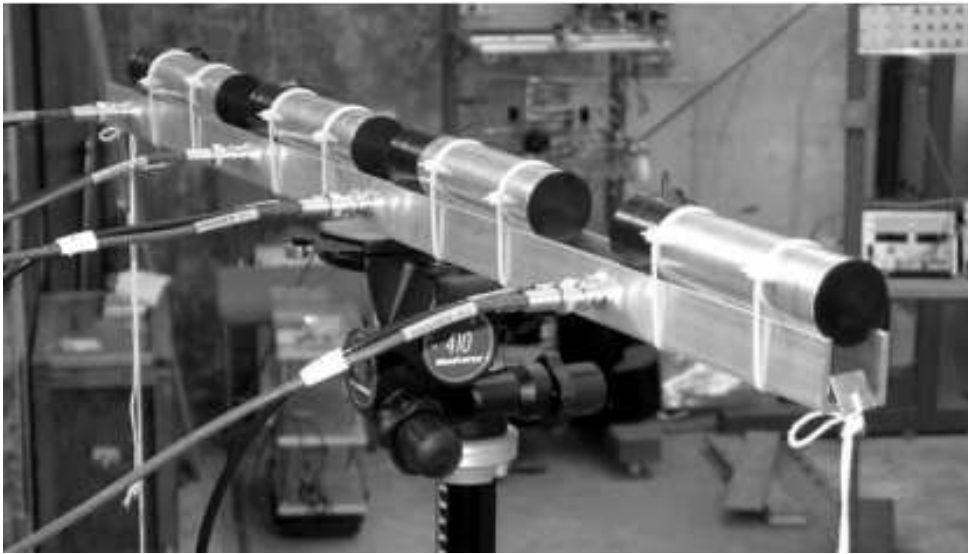
Figure 2.42: Photograph of a typical detector configuration during the 2004 test run at CERN PS. There are four PMT + quartz detector units. Each unit has its own aluminum casting with plastic end cups.
