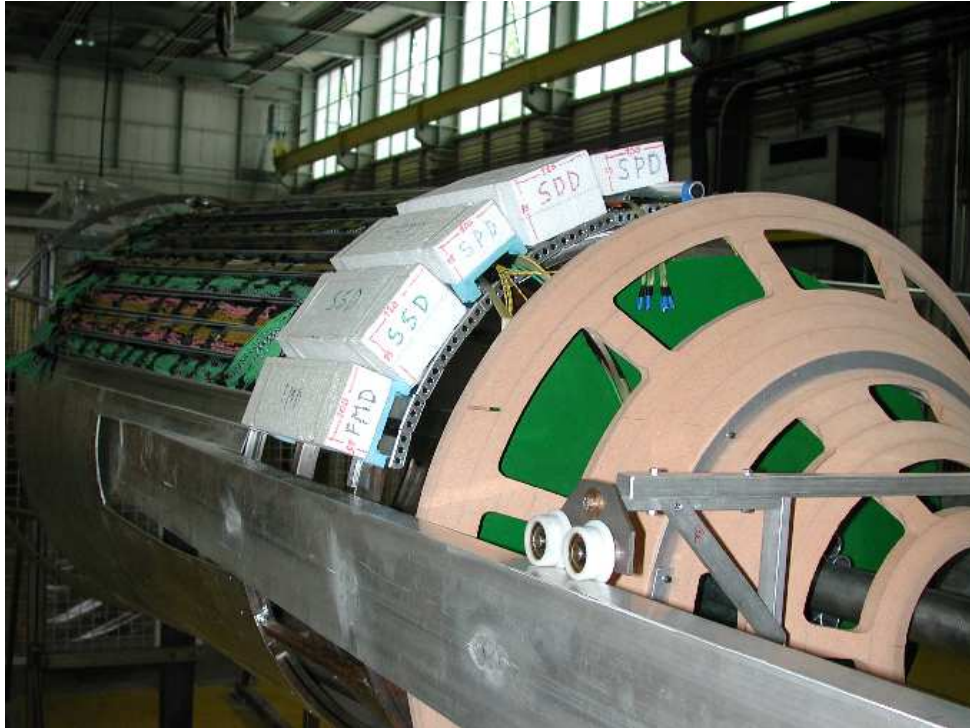
Figure 4.40: Photo of a 1:1 scale model of the ITS and FMD used to study aspects of the mechanical installation and cabling. The space available for patch panels is represented by white blocks.
