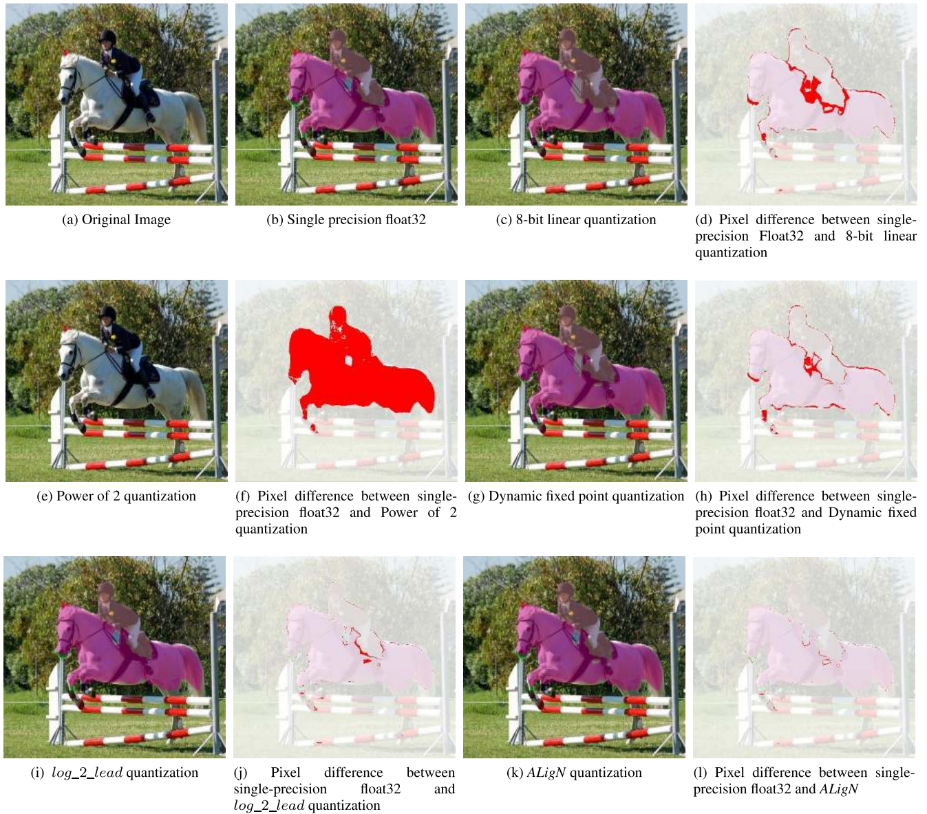
FIGURE 18. Object detection comparison with different quantization schemes using FCN8 [26] network on PASCAL VOC 2012 validation set [27].
