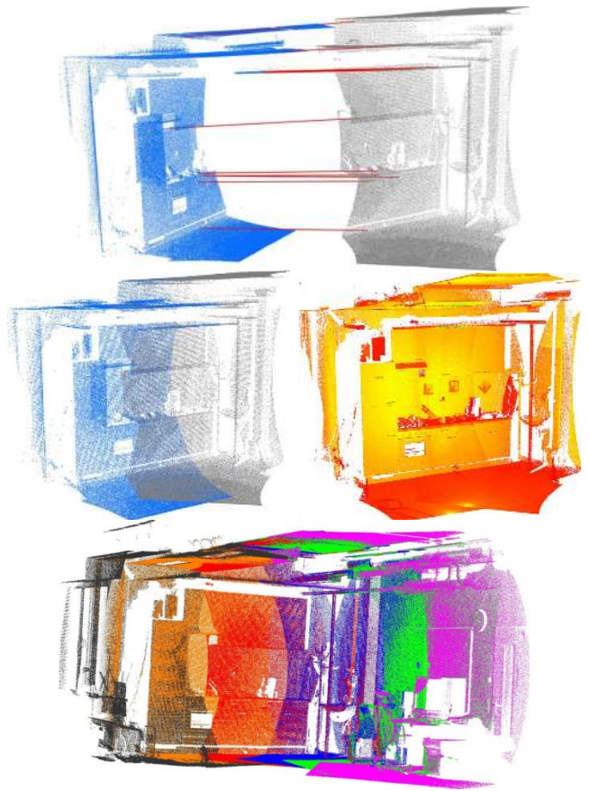
Fig. 2. Aligning 2 scans of a kitchen using persistent feature histograms: corresponding points (top), and computed initial alignment (middle). The final result after registration for a sequence of 5 scans is shown at the bottom.
