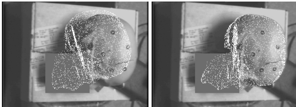
Figure 5.9: An image including an artificial occlusion. White spots denote the pose of the model. On the left is the initial pose, on the right is the final pose.
