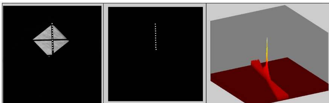
Figure 4.2.3 Rotated ARC image quadrant (left) produces a set of line position estimates seen as white dots. Using the position of the dots, a binary image is created (center). The resulting accumulator space from the binary image yields a fast and accurate line fit to the data as seen in the high sharp spike (right)
