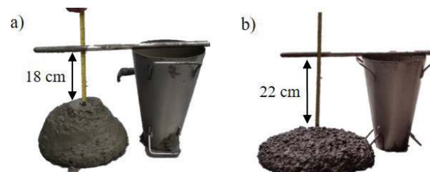
FIGURE 2. Slump test of the mixtures (400 kg/m 3 ): a) OPC (slump = 18 cm) and b) AABC (slump = 22 cm).
