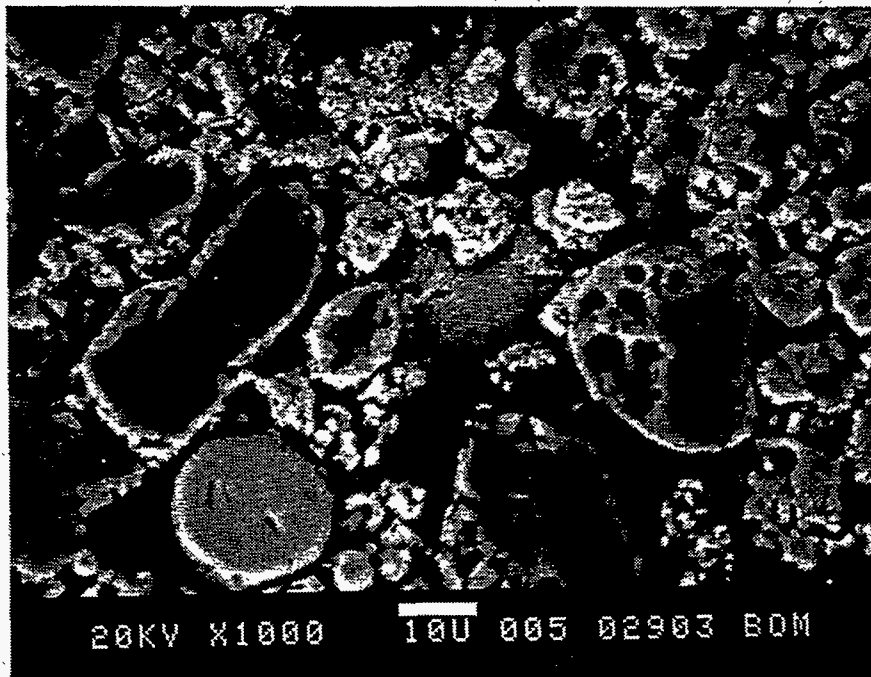
Figure 12.- HydraCo Wood-20 pct Willamette Valley Straw Test Burn: Deposit 008, Backscattered Electron Image of the Center Region of Figure 10, X1,000.
