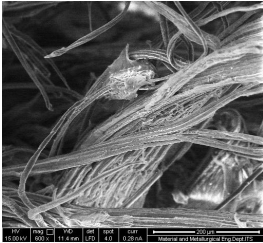
Figure 5 SEM micrographs of bagasse fibers (a) untreated fibers (c) fibers after NaOH treatment for 2 hours (d) fibers after NaOH treatment for 4 hours (e) fibers after NaOH treatment for 6 hours; (b) schematic structure of a natural fiber before and after a treatment [27]
