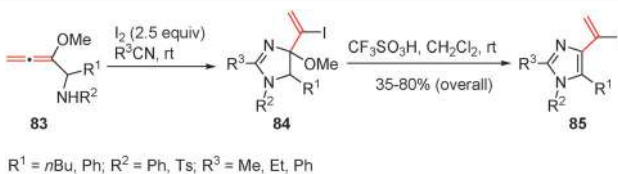
Scheme 30 Synthesis of iodovinyl-substituted imidazole derivatives 85 from allenyl amines 83 and nitriles.
