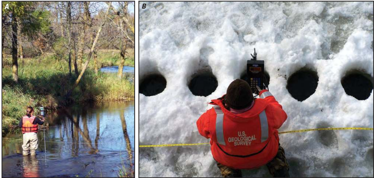
Figure 6. Streamflow measurements at A , the Grindstone River, September 2007, and B , the South Fork Crow River under ice, February 2007.
