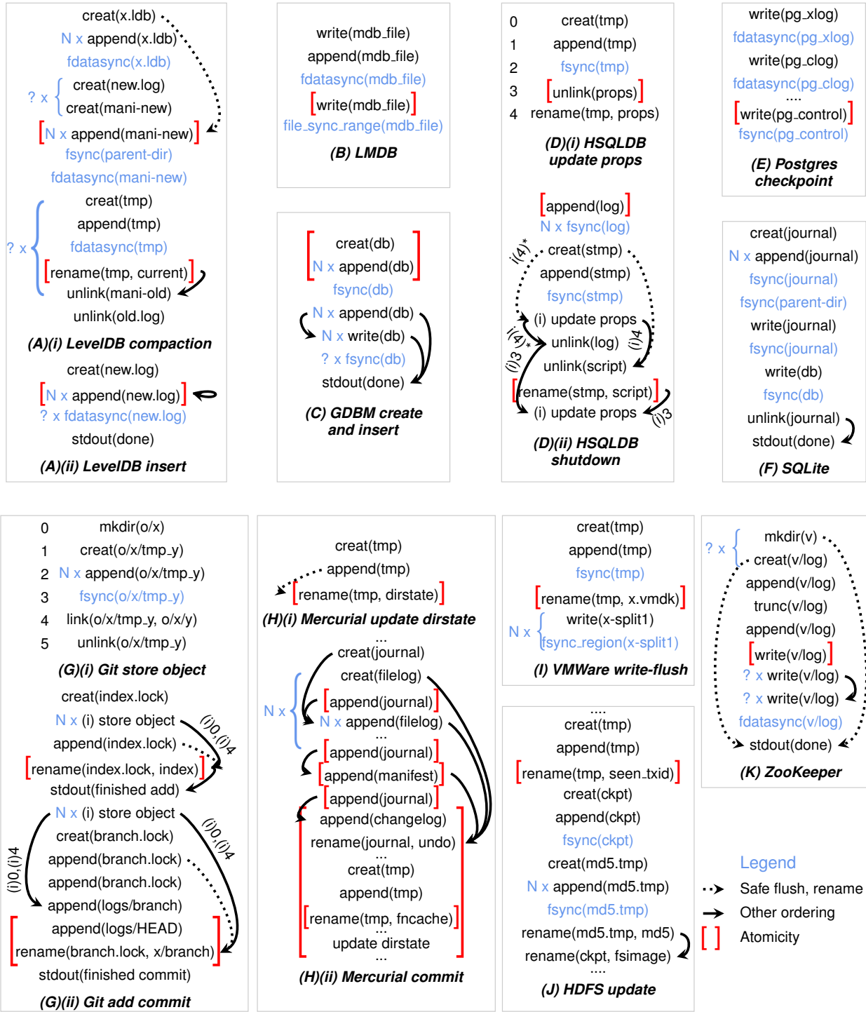
Figure 4: Protocol Diagrams. The diagram shows the modularized update protocol for all applications. For applications with more than one configuration (or versions), only a single configuration is shown (SQLite: Rollback, LevelDB: 1.15). Uninteresting parts of the protocol and a few vulnerabilities (similar to those already shown) are omitted. Repeated operations in a protocol are shown as 'N x' next to the operation, and portions of the protocol executed conditionally are shown as '? x'. Blue-colored text simply highlights such annotations and sync calls. Ordering and durability dependencies are indicated with arrows, and dependencies between modules are indicated by the numbers on the arrows, corresponding to line numbers in modules. Durability dependency arrows end in an stdout micro-op; additionally, the two dependencies marked with * in HSQLDB are also durability dependencies. Dotted arrows correspond to safe rename or safe file flush vulnerabilities discussed in Section 4.4. Operations inside brackets must be persisted together atomically.
