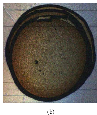
Fig. 3 Proposed device as a humidity sensor: (a) cross section of the proposed device before coating with SnO 2 nanoparticle and (b) photo of drop coated SnO 2 in the top of optical channel waveguide.
