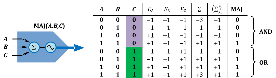
Figure 2. Truth table of the majority gate. The table contains symbol values ( A, B, C ), accompanied complex electric field amplitudes ( E_A, E_B, E_C ), the sum of the electric field amplitudes ( \Sigma ), and the normalized output (\Sigma)_1^0 ; the normalization operation is denoted as (x)_p^0 \equiv px/|x| .
