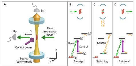
In the setup (Fig. A), we first stored a gate photon in the atomic ensemble, which corresponds to a collective atomic excitation to state |s| (Fig. B). This collective excitation blocks the transmission of source photons through the cavity (Fig. C) and can be retrieved into its original mode (Fig. D). Retrieved gate and
