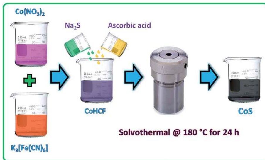
Fig. 1 Schematic of the CoHCF complex preparation and solvothermal decomposition of CoHCF into CoS nanoparticles.
